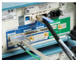
UltraSync connection on instrument with Master role
