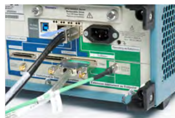
UltraSync connection on instrument with Extension role
